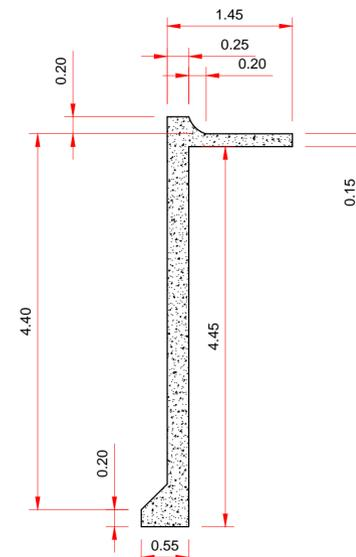
DETALHE MURO - ESC. 1:25
